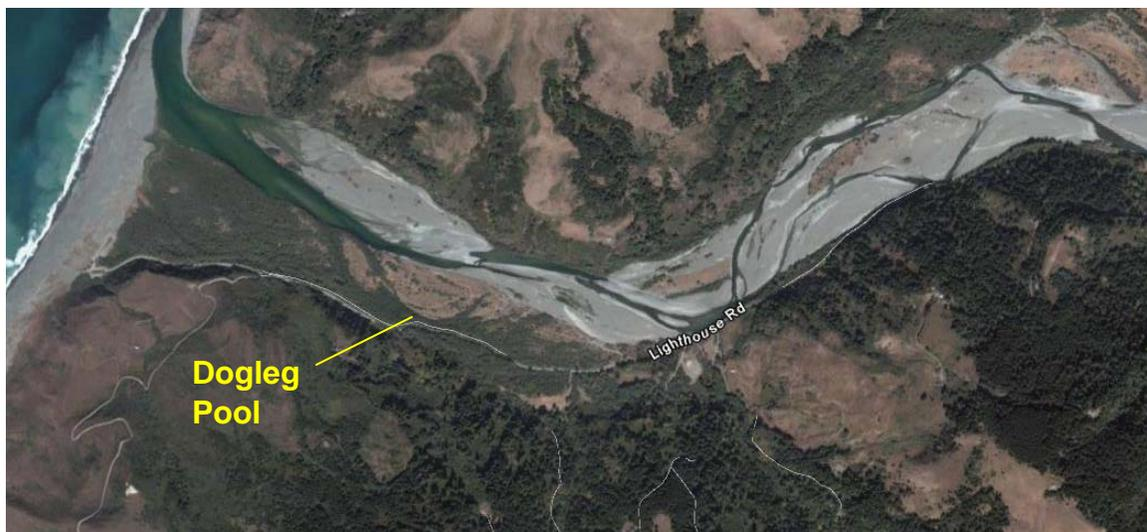
**FIGURE 13)** Aerial photo from July 2007. Note growth the vegetated floodplain near the Dogleg Pool. Vegetation outlines remnant channels well.
