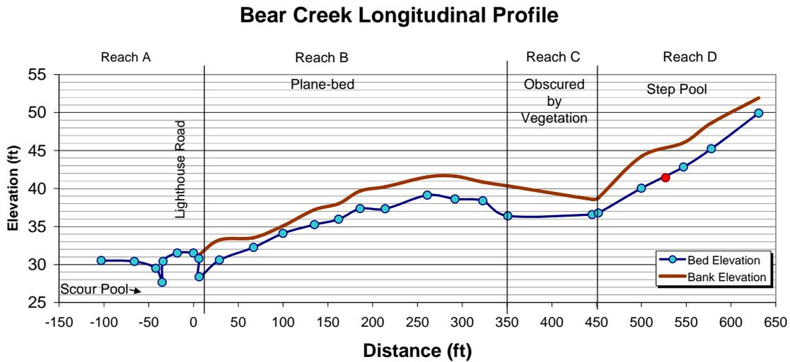
**FIGURE 10)** Longitudinal profile of Bear Creek, showing the variation in bed and bank elevations. Note that the slight decrease in bed height in Reach C. There may be survey errors associated with this depression, although a check point (red dot) surveyed from above suggests that elevations are correct in the profile. Thus the depression appears to be real, and may reflect a backwater zone formed by deposits of coarse sediment in the upper extent of Reach B.
