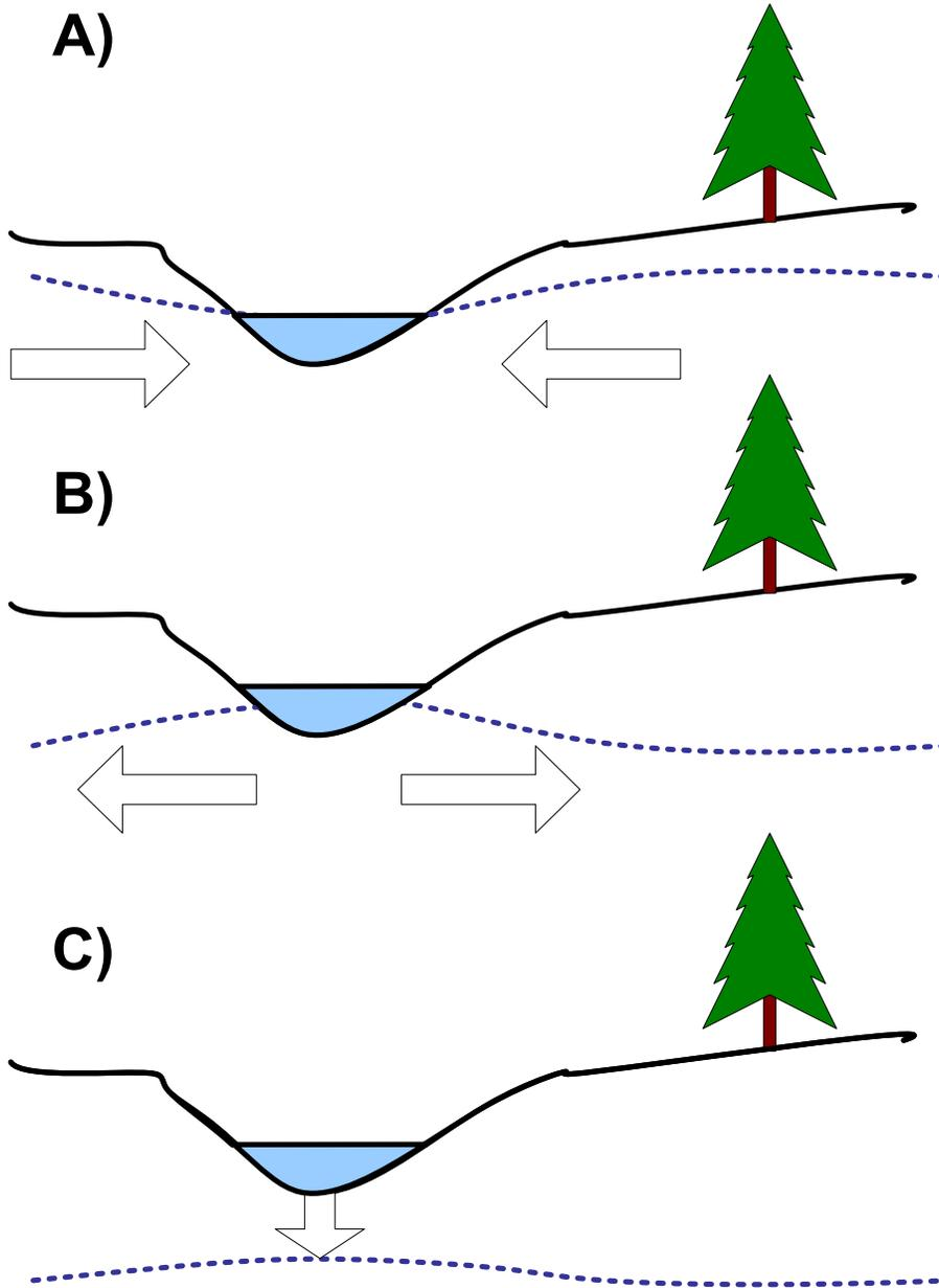
NOTES: Typical flow patterns for groundwater environments; A) gaining streams supported by higher groundwater table surfaces adjacent to the stream; B) losing streams where the stream supplies water laterally and C) losing streams where the stream supplies water vertically.
