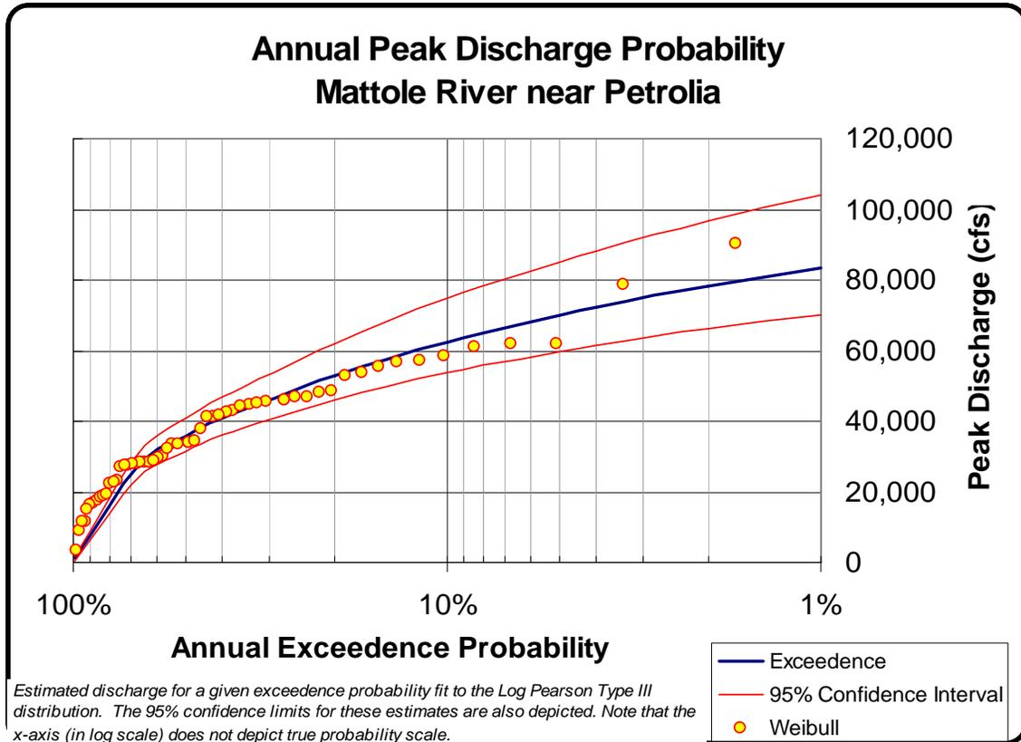
**FIGURE 6)** Peak flow estimates for the Mattole River using the Log Pearson III methodology (USGS Bulletin 17b) and Weibull methodology. Data was provided by the USGS gage for the Mattole River near Petrolia (station 11469000) from 1912 through 2005.
