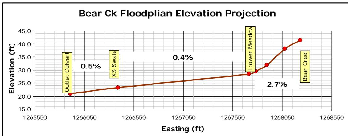
**FIGURE 18)** Projection surveyed points along transect between Bear Creek and the outlet culvert at the west end of the floodplain surface. Survey verifies that a downslope trend exists, satisfying the basic requirement for new channel design. Numbers between stations represent the average downslope gradient.
