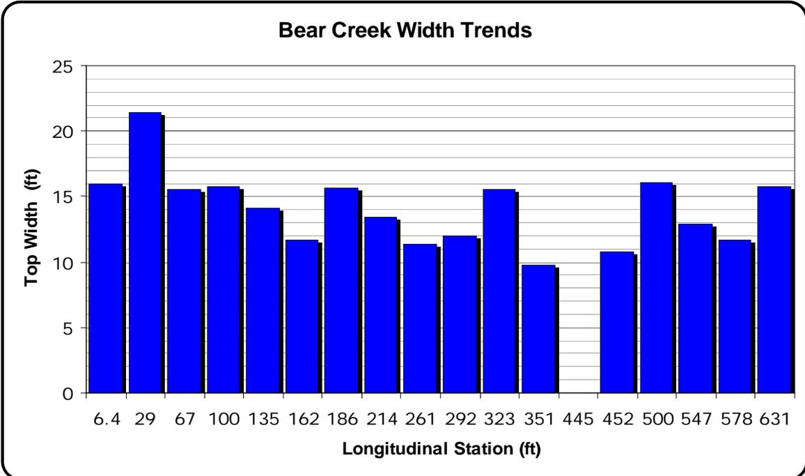
NOTES: Trends in bankfull channel dimensions. Longitudinal station zero is at Lighthouse Road; stations proceed upstream. Note capacity loss at station 67-100, indicating flood risks.
