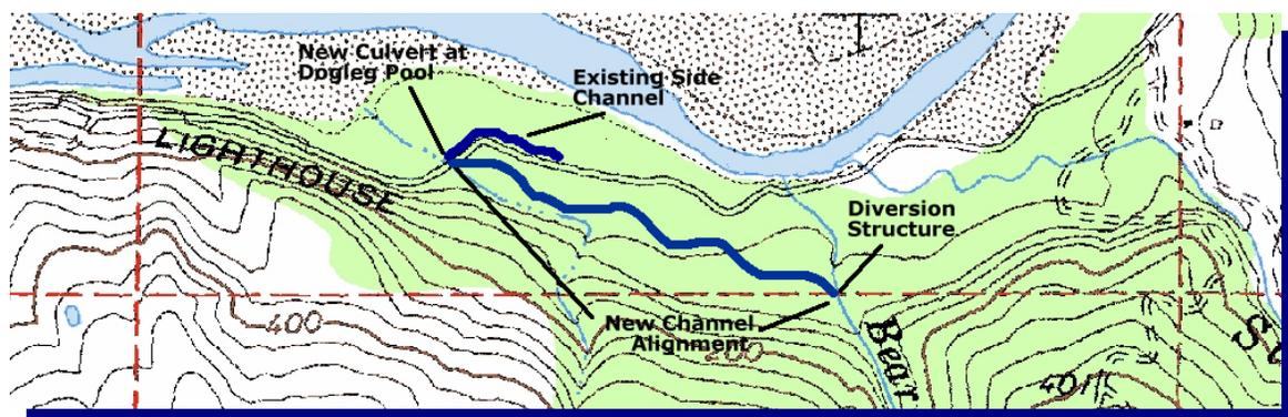
**FIGURE 1)** Conceptual depiction of Alternative 1. Actual channel sinuosity will depend on substrate conditions, channel dimensions, and other characteristics that will be developed during the next phase of design work.
